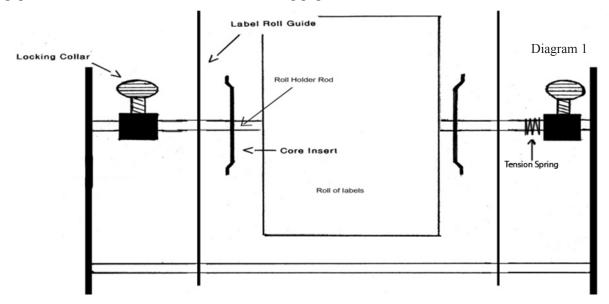
There are two 11" long, 1/16" aluminum roll guides and a tension spring included with the machine. These guides should be placed on either side of the roll of labels between the metal core inserts and the locking collar. The notches on the end of the guide slide onto the chrome rod at the bottom of the machine. Tension spring goes between the right roll guide and the locking collar on the right side of the roll of labels as shown in diagram 1.
